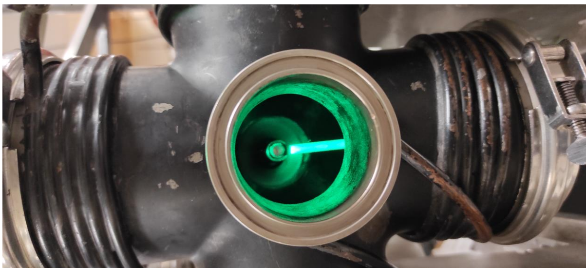
Figure 1 Laser induced fluorescence spectrum of FeH molecule produced in Broida oven
